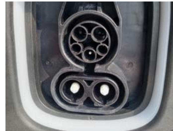
This is on the electric car. Level 2 is with the circular port above. Level 3 will take all ports including the ports below.
